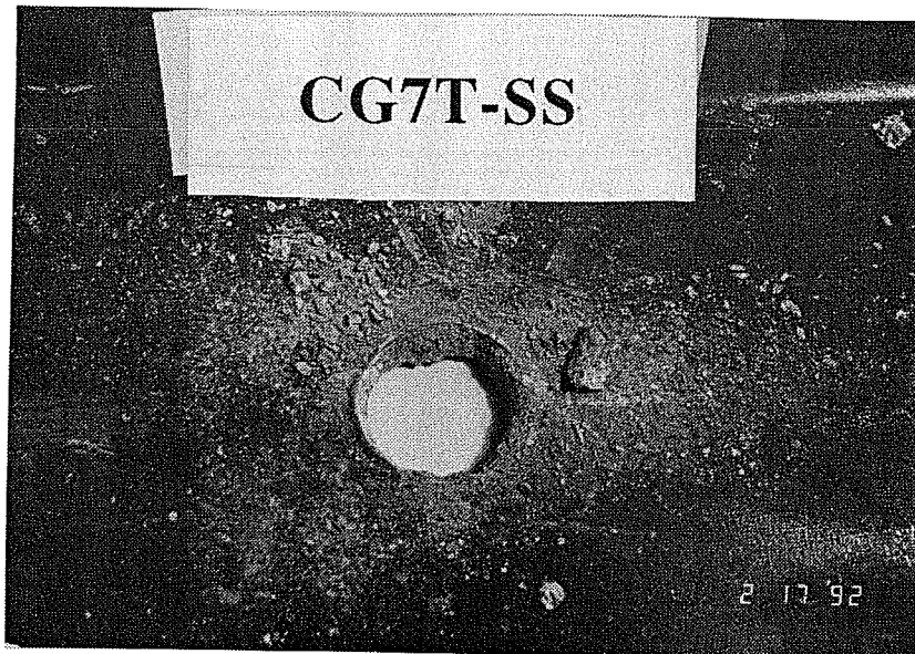
Figure 4.60 Crushing of grout in annulus - Test CG7T-SS
