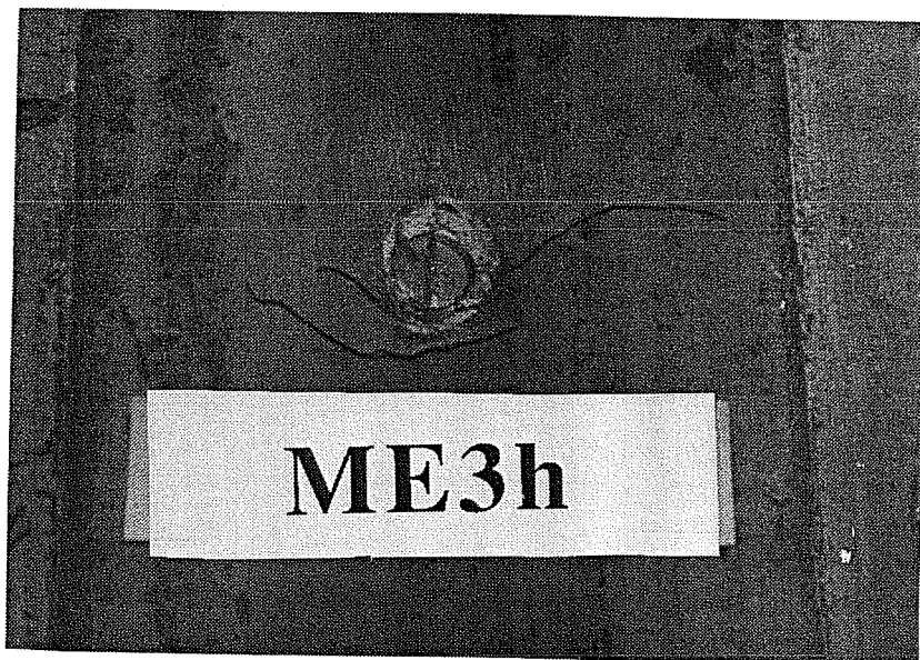
Figure 4.33 Cracking in tension of interface epoxy - Test ME3h
